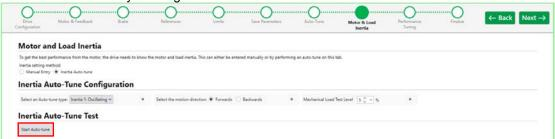
The tool will advise you to close the STO switch to apply 24V to the STO terminal and run the test.
