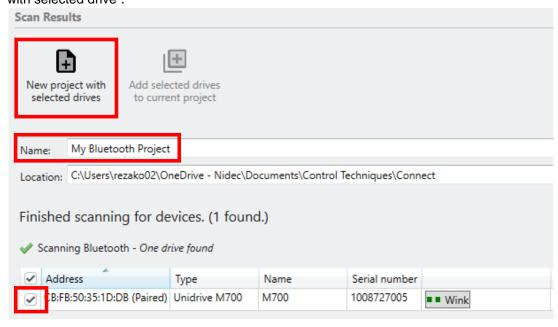
**HINT:** A drive can be identified by using the button which causes the keypad display to flash, this is especially useful in scenarios where multiple drives appear in the list of found devices.
