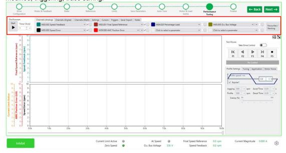
Test move commands – enable the test controls, jog forward / backwards, automatic running as a tuning reference.
