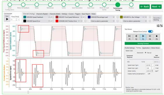
In the previous example trace it can be seen that there is significant speed overshoot caused by the load inertia and default gains. The speed following error shows oscillations when accelerating and decelerating. All of these artifacts can be tuned out easily using "Bandwidth" mode and adjusting the slider control to achieve the desired performance.
