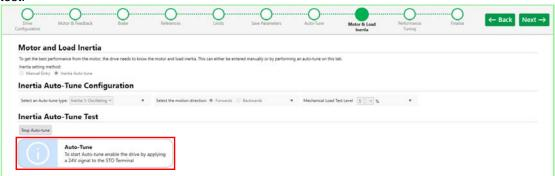
When the test completes, remove 24V from the STO terminal.
