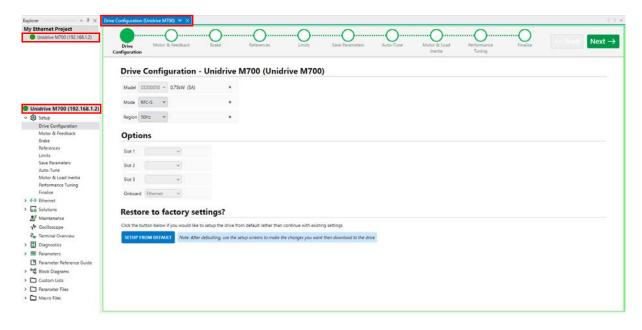
On this page the user can default the drive to remove any previous setup, change the operating mode to match the motor that has been connected to the drive, and select the region e.g. 50Hz or 60Hz.
