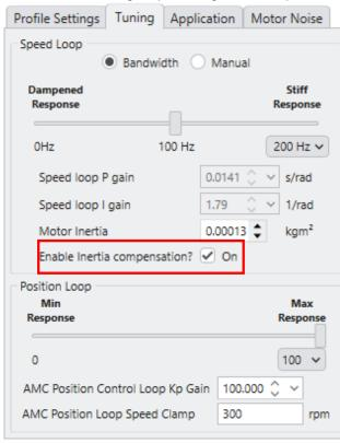
If motor noise induced by the inertia compensation term must be reduced, or the amount of inertia compensation must be increased to further improve the following error, select manual speed loop tuning to disconnect the inertia value from the speed loop gain setting. Then decrease the inertia value to reduce motor noise or increase the inertia to increase the output of the inertia compensation.
