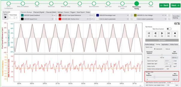
If the P Gain needs to be pushed above 100 the range can be increased using the following control:
