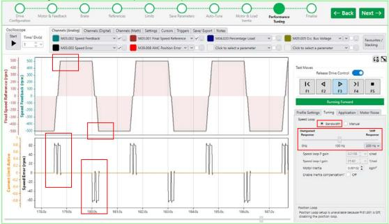
From the previous trace it can be seen that there is no significant speed overshoot, the speed following error isn't oscillating, and the drive isn't going into current limit.
