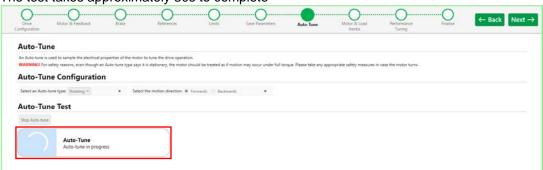
When the test completes, the drive must be disabled by removing 24V from the STO input.
