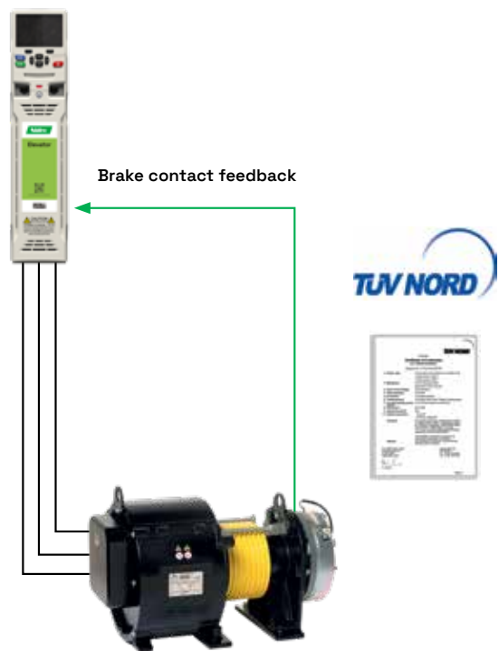
TÜV certified Brake Contact Monitoring functions on the Elevator Drive E300
